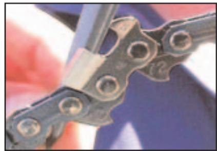
You can see how the side bevel on the file cuts the "v" to the point and the complete side channel of the tooth.
