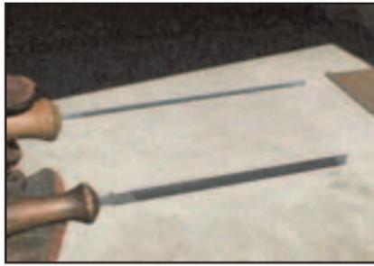
Two chisel bit file types are available from PFERD. A six-sided triangular and a six-sided flat version.
